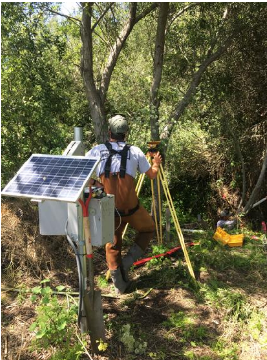
Restoration Coordinator Seamus Land surveys the Oso Flaco Creek channel cross section for the RCD stream gauging project.
